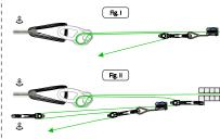
The Wafer 2.0, when combined with roller carabiners, weblocks, and soft releases, can be used to tension a slackline in a number of configurations. Above we have 2 common configurations that are often used.
